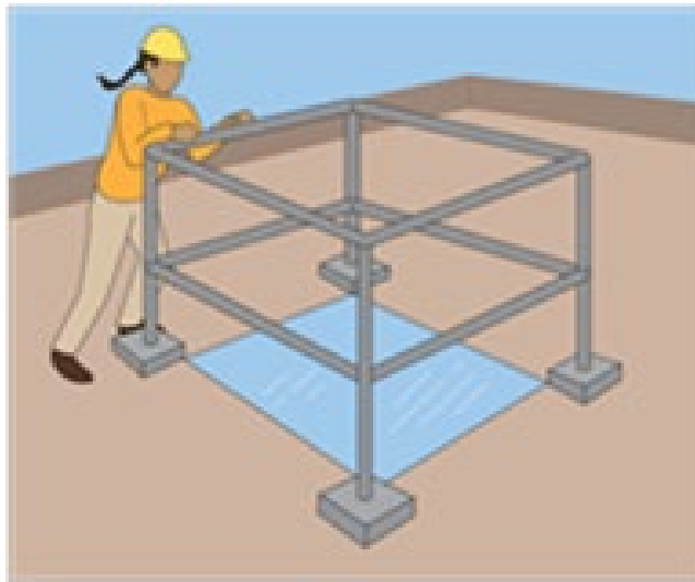
Figure 1 Guardrails should be used around floor openings
