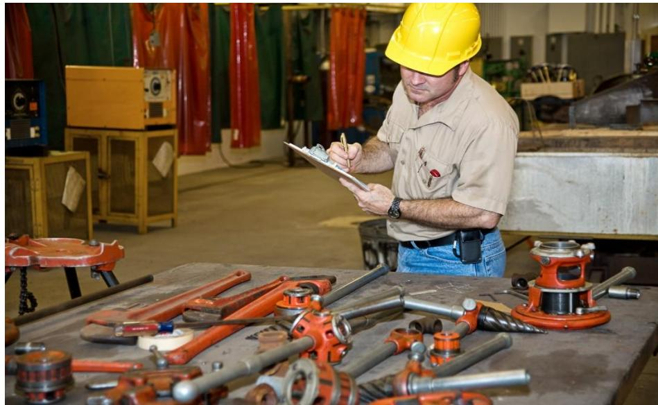
Today's safety talk focuses on **manual hand tools** — not electric or pneumatic — such as **hammers, screwdrivers, chisels, and wrenches**. These are common tools, but they can cause serious injuries if they're not in good shape.
